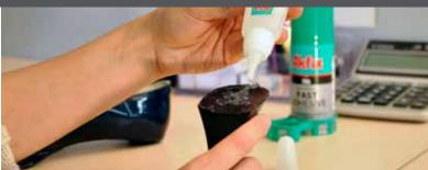
Adhesive set which consists of high viscosity cyanoacrylate adhesive and activator.
