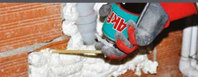
Single-component, moisture-curing and self-expanding aerosol polyure-thane foam. It is designed for easy dispensing through the straw adapter included with each can. It does not contain any propellant gases that are harmful to the ozone layer.
