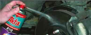
Powerful cleaning fluid is used to remove oil, grease, dirt and dust from brakes and clutches, aiding in the elimination of brake squeal and clutch slip caused by glazing and contamination. Brake cleaner helps brakes last
